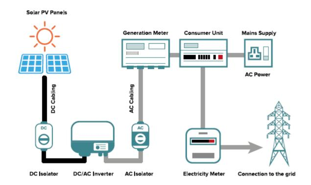
Solar panels are typically attached to the roof of a home, although they can be integrated into the roof instead. When light shines on the panels, this energy is converted into direct current (DC) electricity. The greater the intensity of the light, the greater the flow of electricity
